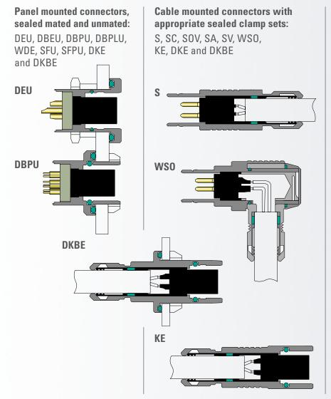
Cable mounted connectors with appropriate cable assembly solution:
