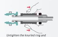
pull the outer sleeve to unlock
